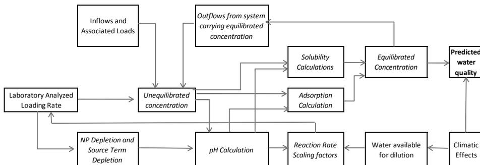
Figure 1 Overview of water quality algorithm included in the model
