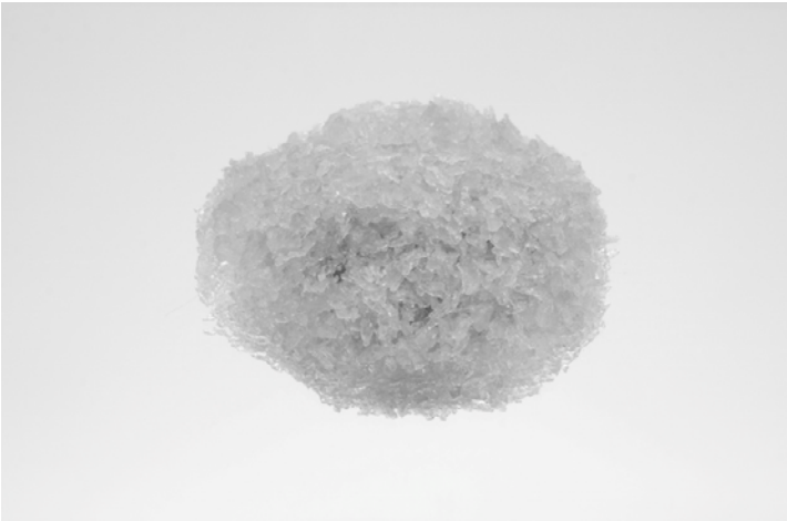
Figure 2 Melanterite obtained from the hydrometallurgical/UV processing of the coal tailing
