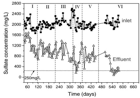
**Figure 3.** Sulfate concentration during the sulfate reduction in a UASB reactor. Experimental conditions: (I) OLR = 3.48 kg/m<sup>3</sup>.d; (II) OLR = 4.87 kg/m<sup>3</sup>.d; (III) OLR = 3.55 kg/m<sup>3</sup>.d; (IV) OLR = 4.65 kg/m<sup>3</sup>.d; (V) OLR = 5.89 kg/m<sup>3</sup>.d; (VI) OLR = 5.04 kg/m<sup>3</sup>.d.
