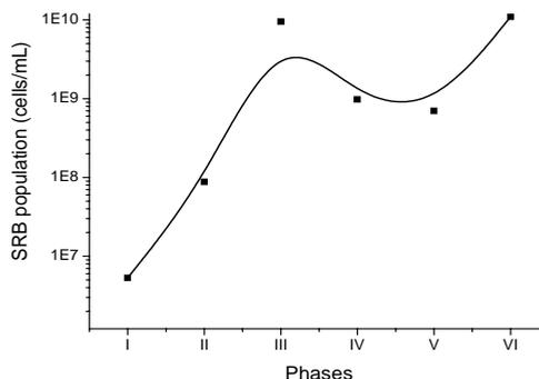
**Figure 1.** Monitored BRS population in the UASB reactor. (I) OLR =  $3.48 \text{ kg/m}^3\text{.d}$ ; (II) OLR =  $4.87 \text{ kg/m}^3\text{.d}$ ; (III) OLR =  $3.55 \text{ kg/m}^3\text{.d}$ ; (IV) OLR =  $4.65 \text{ kg/m}^3\text{.d}$ ; (V) OLR =  $5.89 \text{ kg/m}^3\text{.d}$ ; (VI) OLR =  $5.04 \text{ kg/m}^3\text{.d}$ .
