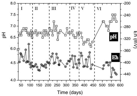
**Figure 2.** Variation on pH and Eh during the UASB reactor performance. Experimental conditions: (I) OLR = 3.48 kg/m<sup>3</sup>.d; (II) OLR = 4.87 kg/m<sup>3</sup>.d; (III) OLR = 3.55 kg/m<sup>3</sup>.d; (IV) OLR = 4.65 kg/m<sup>3</sup>.d; (V) OLR = 5.89 kg/m<sup>3</sup>.d; (VI) OLR = 5.04 kg/m<sup>3</sup>.d.
