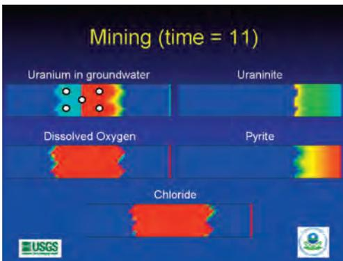
**Figure 3** Five-spot ISR mining with oxygen and carbon dioxide. Flow is from left to right.
