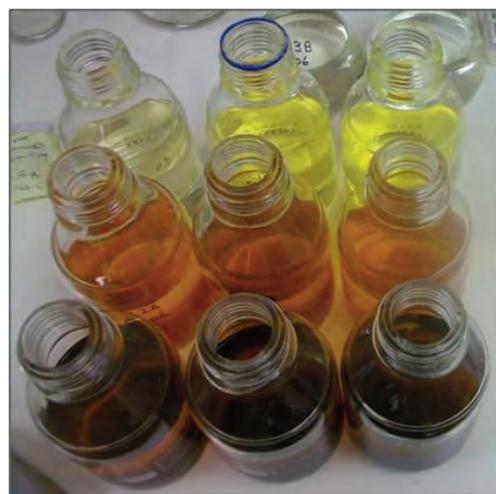
**Figure 2** Dissolved steam coal condensate in solvent (time increasing – horizontal, temperature decreasing – vertical).
