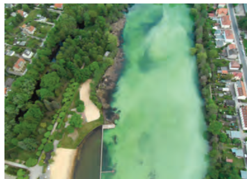
Figure 7 Aerial photograph showing the distribution of alkalinity after 40 minutes
