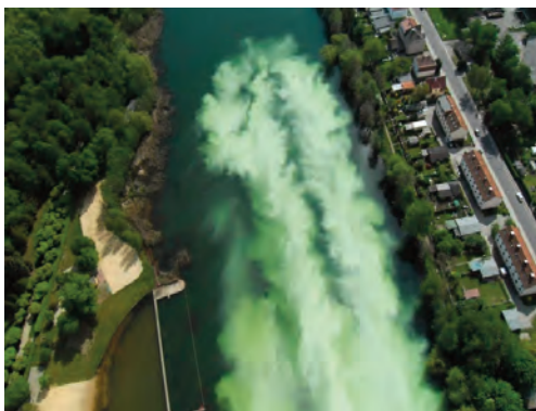
Figure 6 Aerial photograph showing the distribution of alkalinity after 10 minutes.
