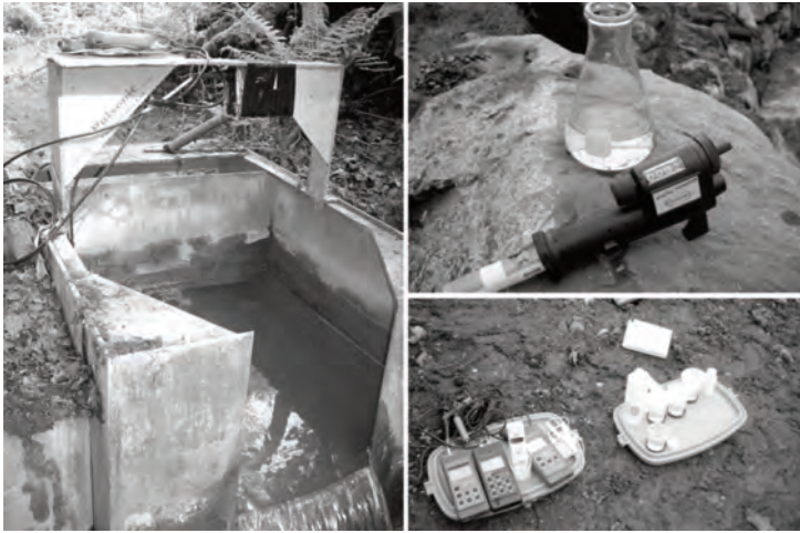
Figure 2 Examples of changes to monitoring requirements (left is a rectangular weir with a datalogger, top right is a digital titrator, bottom right are some on-site testing equipment).
