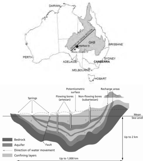
**Figure 1** The Great Artesian Basin of Australia (cross-section from <http://www.gabcc.org.au>)
