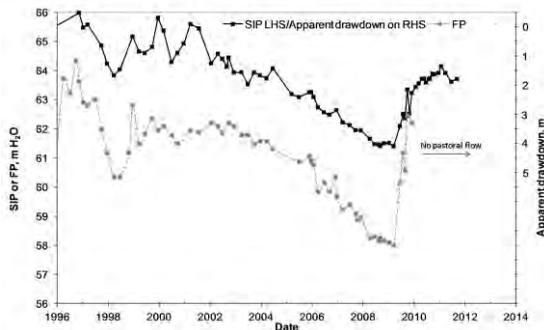
**Figure 3** Shut-in Pressure (SIP), Flow Pressure (FP) and Apparent Drawdown in Jackboot Bore
