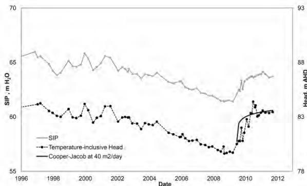
**Figure 4** Shut-in Pressure (SIP) and Temperature-inclusive Head
