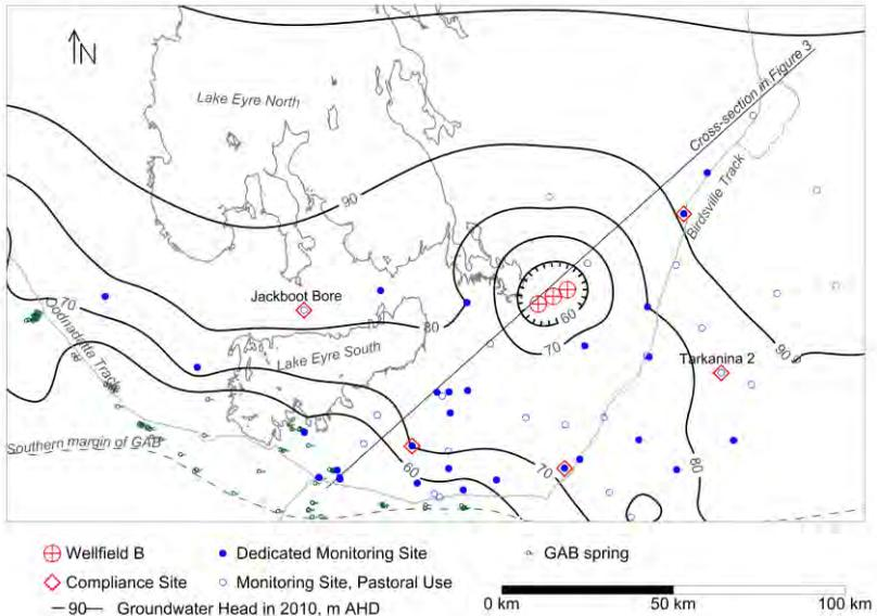
**Figure 2** Wellfield B, monitoring and compliance sites
