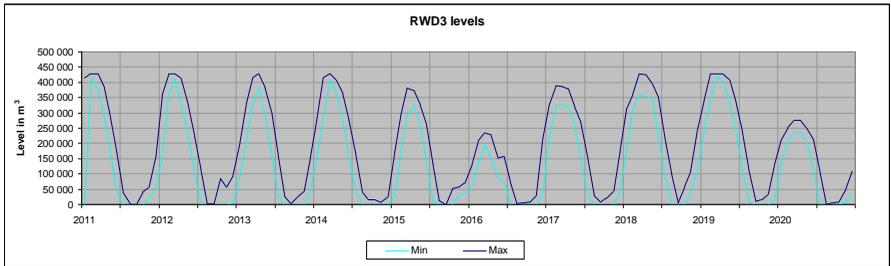
**Figure 2** Simulated levels of the Tailings Return Water Dam 3
