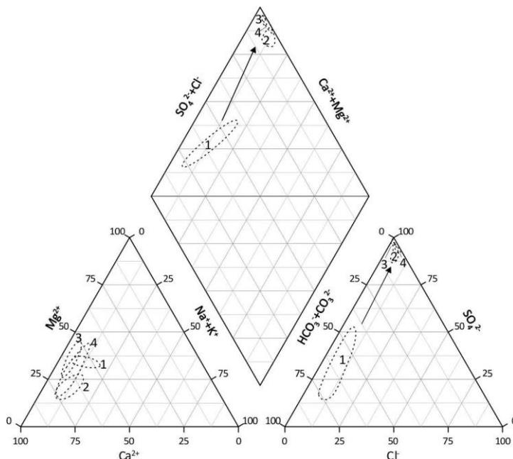
**Figure 2.** The Piper diagram showing the chemical composition of surface and groundwater in the Mitek catchment. 1 – water from the upper parts of Mitek stream (P1), 2 – mine water outflow from the mine shaft (P2), 3 – mine water outflow from the foot of the dump (P3), 4 – water from the mouth of the Mitek stream (P4).
