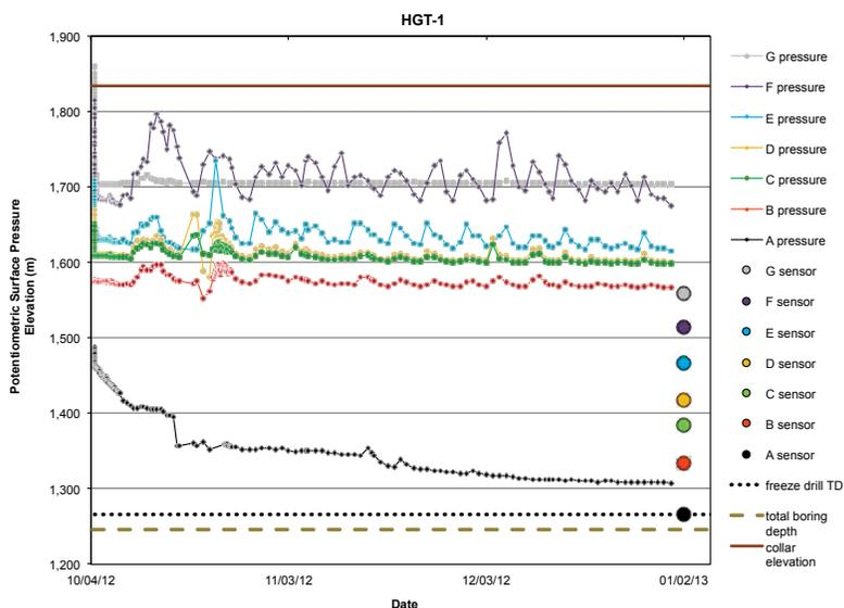
**Figure 4** Potentiometric surface pressure represented as total elevation head in HGT-1. Symbols shown on the right side of the graph correspond with VWP sensor installation depths in HGT-1. The average total depth of the freeze wells drilled for construction of the shaft 15 m south of HGT-1 is indicated by "freeze drill TD." The final drilled depth of HGT-1 is indicated by "total boring depth".
