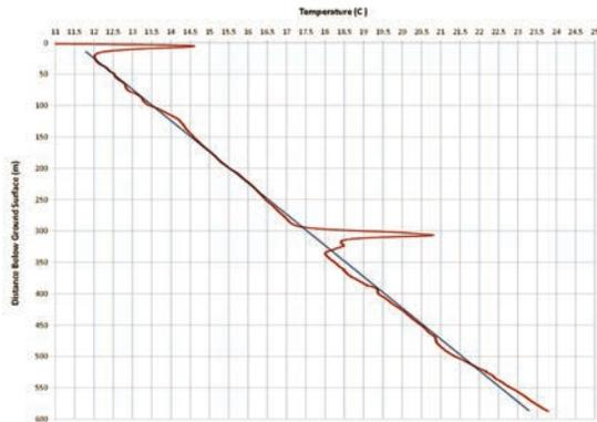
**Figure 2** Average temperature in HGT-1 from 19:47, 12 December 2012 to 00:02, 13 December 2013. The red line is measured average temperature. The blue line is a visually fit straight line, for comparison.
