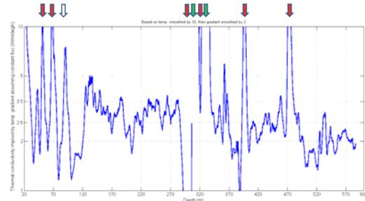
**Figure 3** Implied thermal conductivity of substrate in HGT-1 based on temperature profile of 12 December 2012 (W/m/K).
