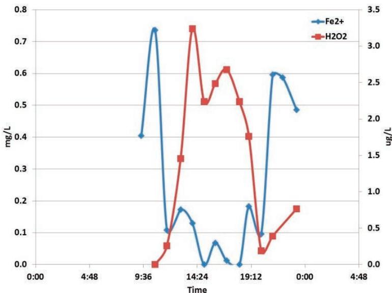
Fig. 2 Ferrous iron is consumed in the photo-Fenton reaction.
