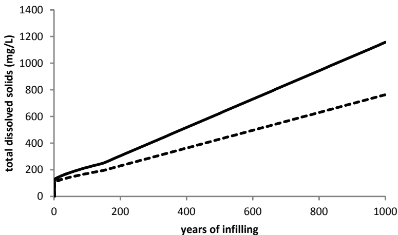
Fig. 5 Pit lake total dissolved solid concentration (mg/L) as a function of time for a 457 m deep, filling to 305 m deep over \approx 150 years, groundwater quality of 100 mg/L at 50 % runoff with a runoff quality of 500 mg/L and pit acreages of 202 ha (---) and 404 ha (—) respectively.
