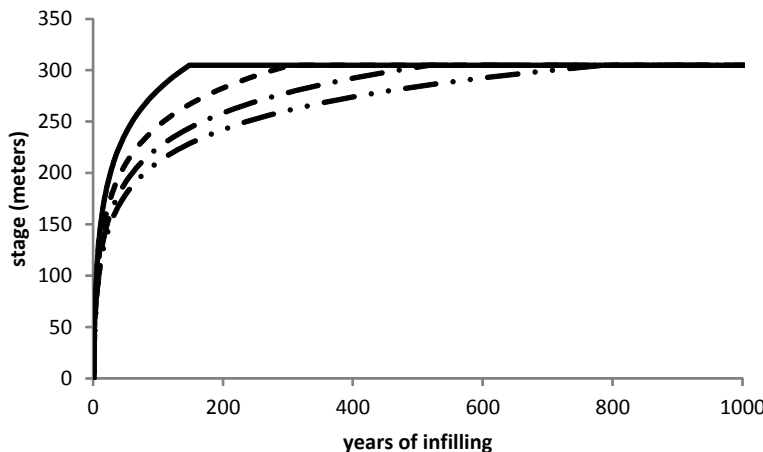
Fig. 2 Time – stage relationship at 202 ha pit, 457 m deep, filling to 305 m deep over ≈ 150(—), ≈ 300(---), ≈ 500(- · - ·), and ≈ 800(- · · -) year periods.
