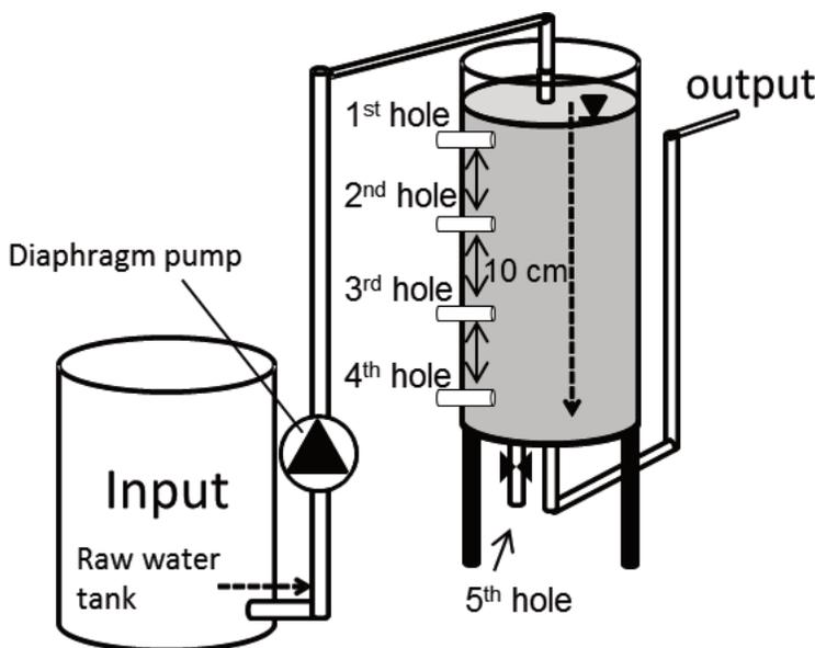
**Fig. 1** A schematic diagram of the setup for continuous treatment test with anaerobic bioreactor.
