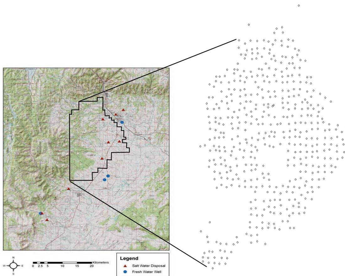
**Fig. 2** Map showing the locations of the four shallow freshwater wells, nine SWD wells, and the wells in the Drunkards Wash gas field used in the structural analysis.
