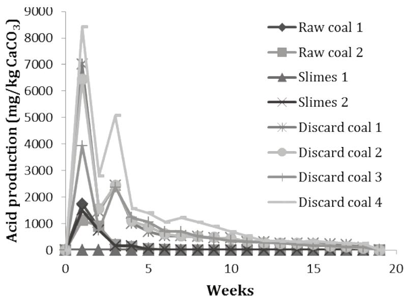
**Fig. 3** Rate of acid generation of samples during phase 2 column leaching test.
