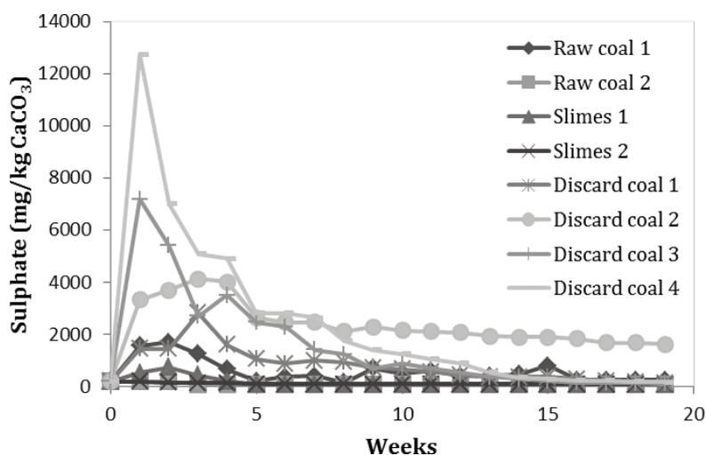
**Fig. 4** Rate of sulphate generation of samples during phase 2 column leaching test.
