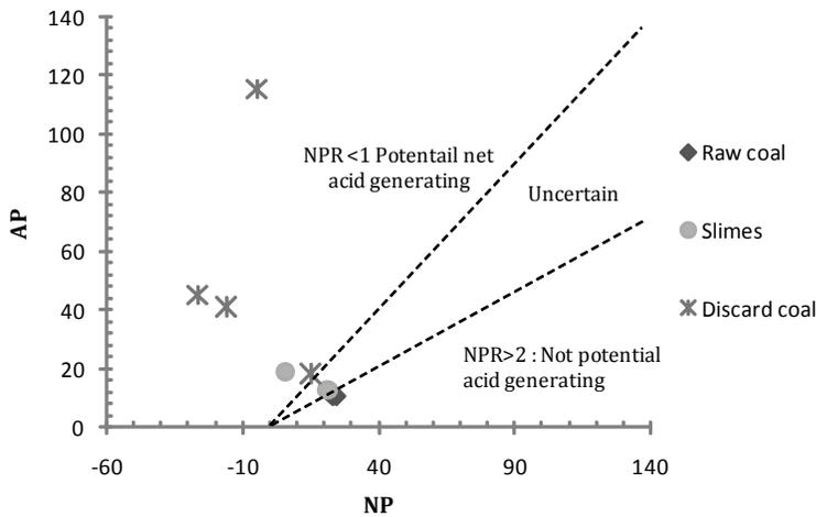
**Fig. 2** Acid potential and Neutralisation potential graph indicating areas of potential acid generating, uncertain range and potential non-acid generating.
