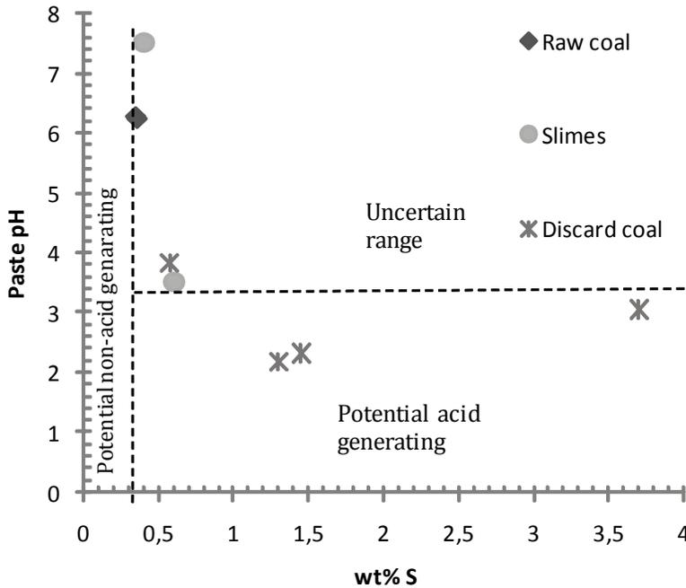
**Fig. 1** Paste pH vs wt % S indicating areas of potential acid generating, uncertain range and potential non-acid generating.
