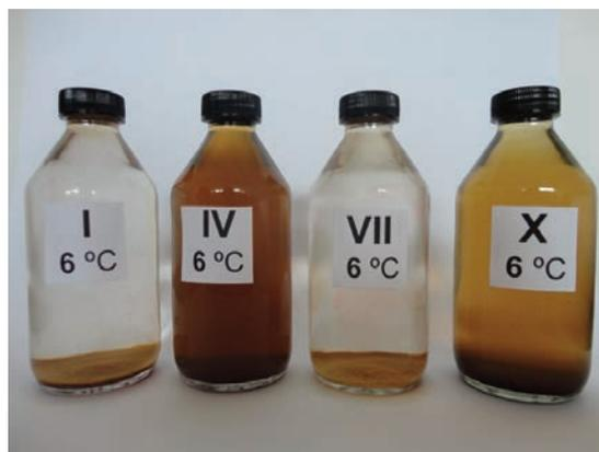
**Fig. 1** Tests incubated at 6 °C, I and VII with negative SRB development in 35 days, IV and X with a very slowly growth starting from 30 and 25 respectively.
