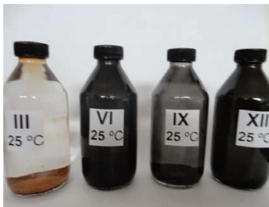
**Fig. 2** Tests incubated at 25 °C, III with negative SRB development in 35 days and XII with a fast SRB development in less than 1 day, depending on sulphate and organic nutrients availability.
