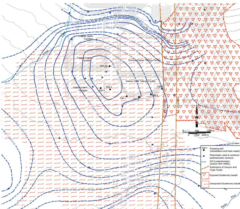
**Fig. 2** Potentiometric contours (based on end of 2012 water levels), extent of exposed and unexposed Quaternary basalt, and aeromagnetically-inferred extensions of the Canyon and Virgin Faults. Note that the contour interval changes in the northern portion of the area shown.
