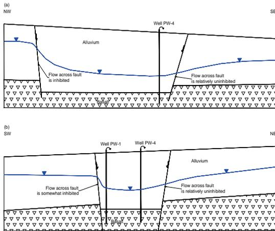
**Fig. 3** Conceptual cross-sections parallel to groundwater flow resulting from the pumping wells (a) and perpendicular to flow (b). Note how fabric developed in alluvium during faulting as well as juxtaposition of different facies across faults creates slightly lower K zones along some faults, but not others. Vertical scale is exaggerated.
