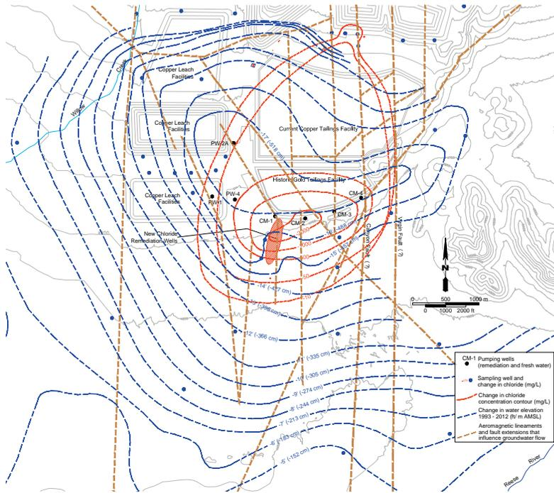
**Fig. 4** Change in water elevation contours from 1993 to end of 2012, and change in chloride concentration contours (1993–1998 vs. 2010–2012 [mg/L]). Key aeromagnetic lineaments that are interpreted to represent faults that have created zones of varying conductivity, and geophysically-inferred extensions of mapped faults that also act as hydrologic boundaries are shown, along with the area selected for replacement remediation wells.
