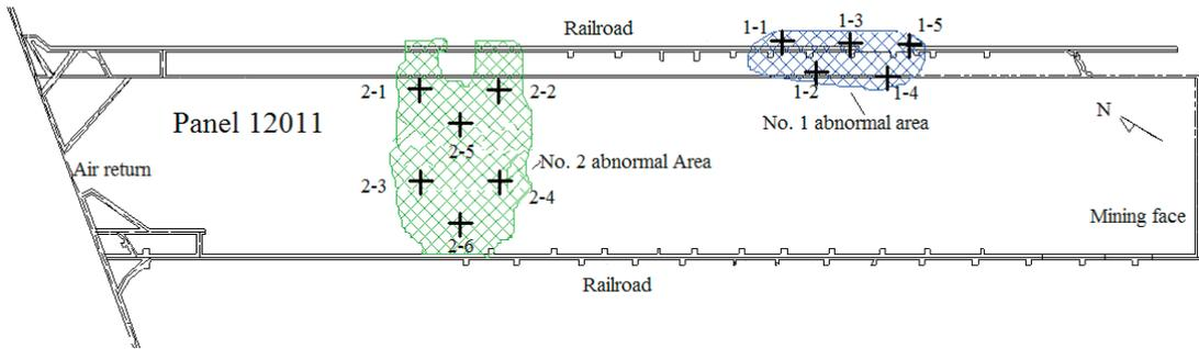
Fig. 4 Location of two abnormal water areas and grouting boreholes
