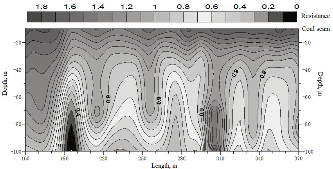
Fig. 6 Apparent resistivity of vertical detection of No. 1 abnormal water area
