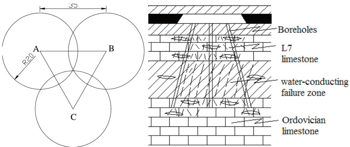
Fig. 5 Grouting borehole design. (a, left) plane view; (b, right) cross section view
