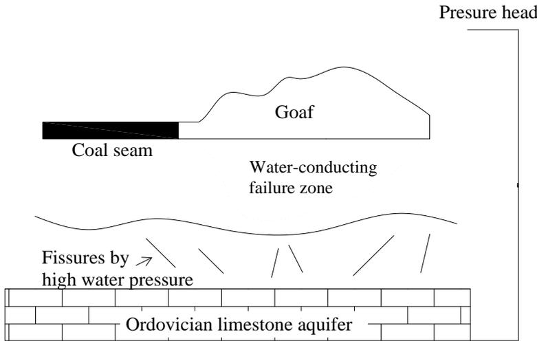
**Fig. 1** Sketch of water-conducting failure zone caused by coal mining
