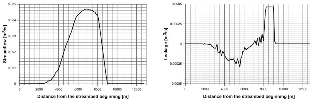
**Fig. 7** Streamflow (left) and leakage between the Stream B and the aquifer (right) in dewatering conditions, upstream of the open pit
