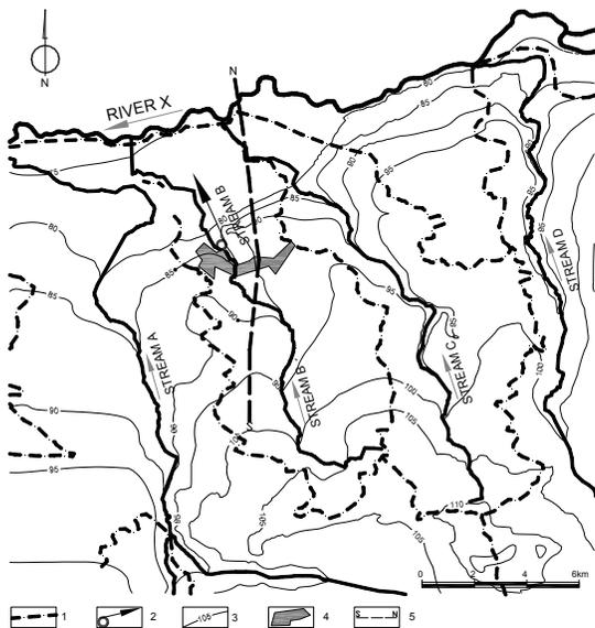
**Fig. 1** Hydroisohypses of the water table quaternary aquifer. Explanations: 1 – watershed, 2 – mine water discharge direction, 3 – hydroisohypses, 4 – open pit area, 5 – hydrogeological cross-section
