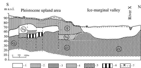
**Fig. 2** The hydrogeological cross-section through the deposit area (S–N). Explanations: 1 – fine and medium sands, 2 – clays, 3 – silts, 4 – argils, 5 – marls, 6 – deposit, 7 – quaternary water table in natural conditions, Q – Quaternary; Ng – Neogene; Cr – Cretaceous
