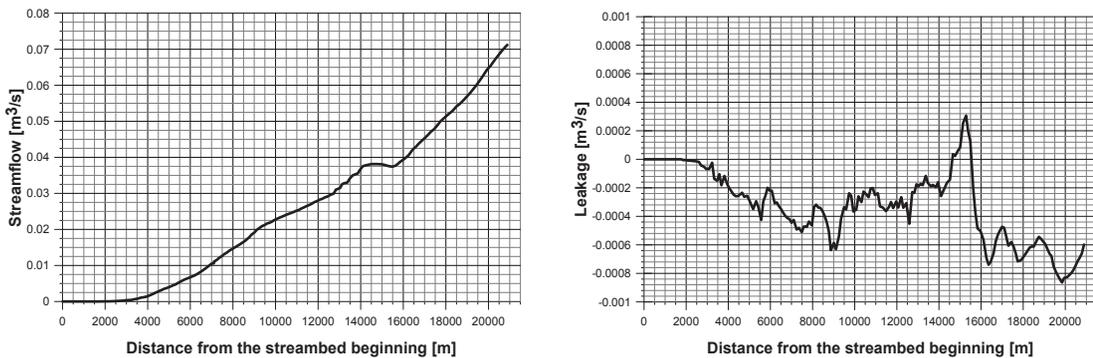
**Fig. 3** Streamflow (left) and leakage between the Stream B and the aquifer (right) in natural condition
