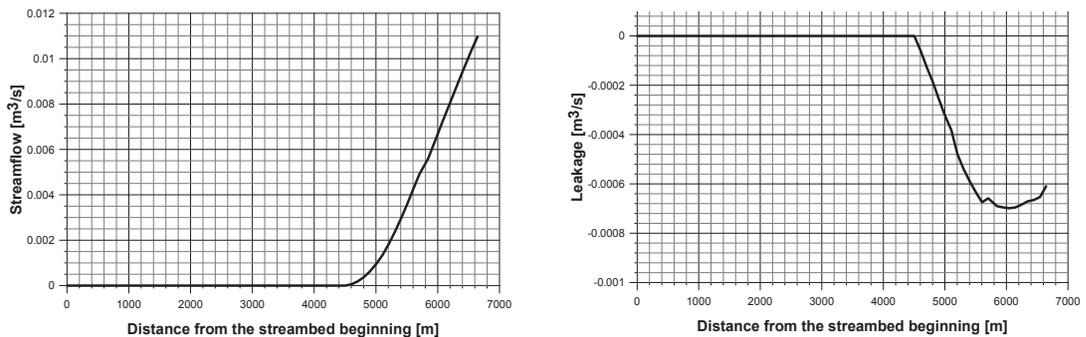
**Fig. 5** Streamflow (left) and leakage between the Stream B and the aquifer (right) in dewatering conditions, downstream of the open pit without mine water discharge
