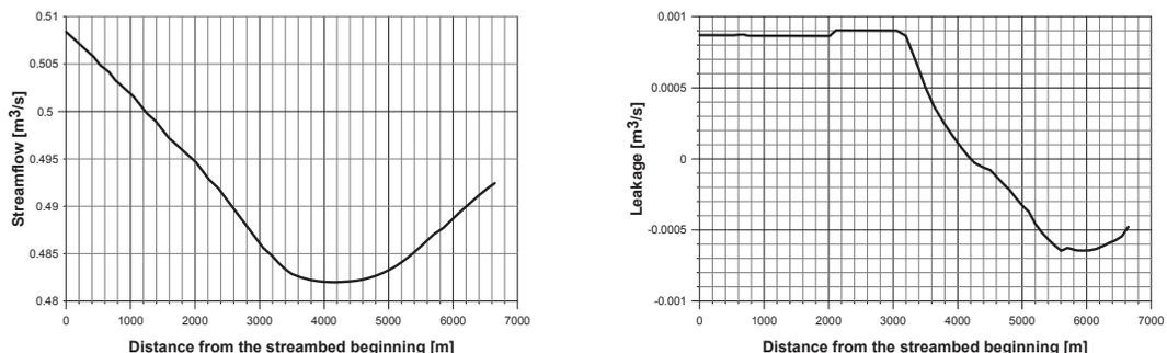
**Fig. 6** Streamflow (left) and leakage between the Stream B and the aquifer (right) in dewatering conditions, downstream of the open pit with mine water discharge  $0.5 \text{ m}^3/\text{s}$
