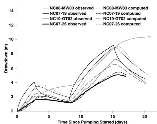
**Fig. 3** NCC model observed versus simulated drawdown for first pumping test data set.
