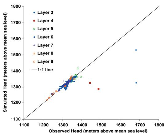
**Fig. 2** Observed versus model-simulated steady-state hydraulic heads.
