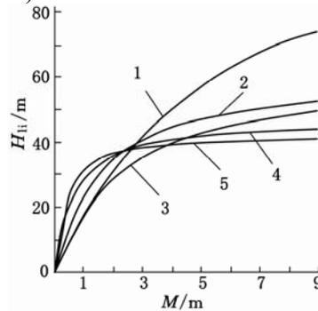
*Fig.1 Curve diagram of coal mining method and water-conducting fracture zone height*
