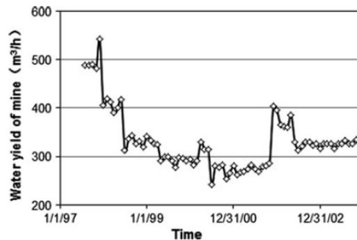
Fig.1 Temporal variation in the rate of water yield of a mine in Anhui, China
