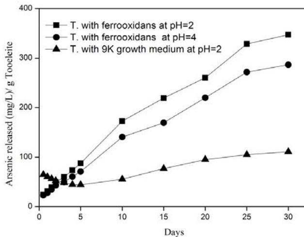
**Fig. 4** Arsenic released from tooeleite with time under ferrooxidans culture and medium at pH=2 and 4
