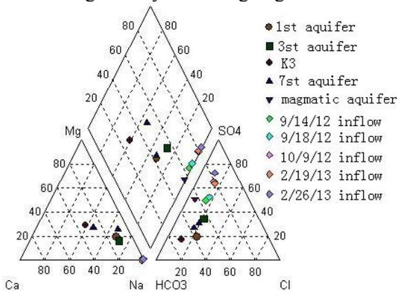
Fig. 6 Piper figure of water quality of each aquifer and working face 8101 in Wolonghu Coal Mine
