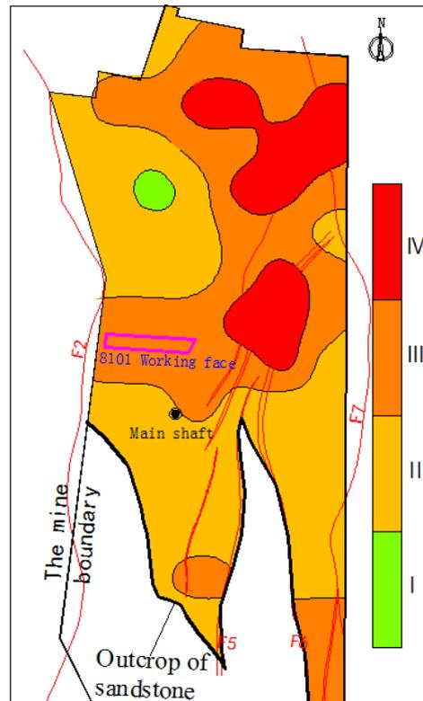
Fig. 1 Section of water abundance of K<sub>3</sub> sandstone aquifer
