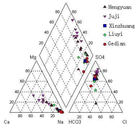
Fig. 7 Piper figure of water quality of sandstone water in adjacent coal mines
