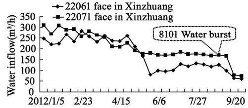
Fig. 3 The comparison diagram of the change of water inflow in 22061 and 22071 face
