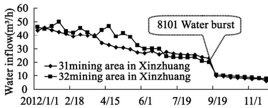
Fig. 4 The comparison diagram of the change of water inflow in 31 and 32 mining area
