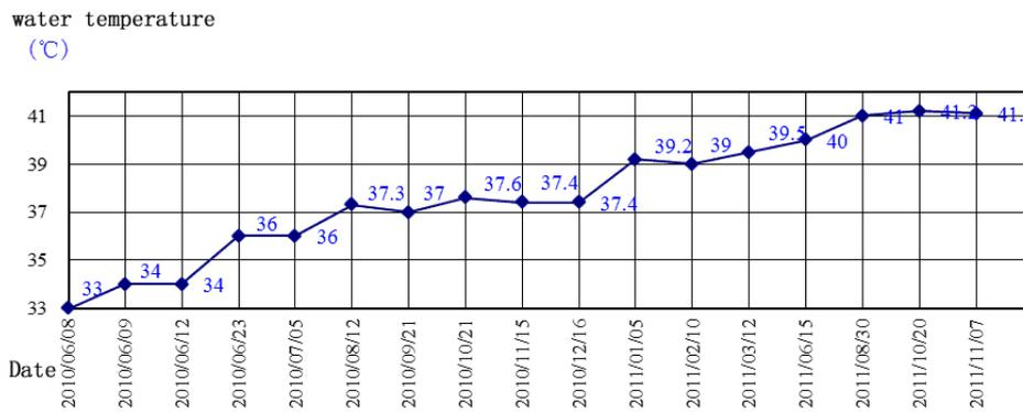
**Fig. 3** Water temperature change curve of the water inrush points in Roadway II5<sub>1</sub>
