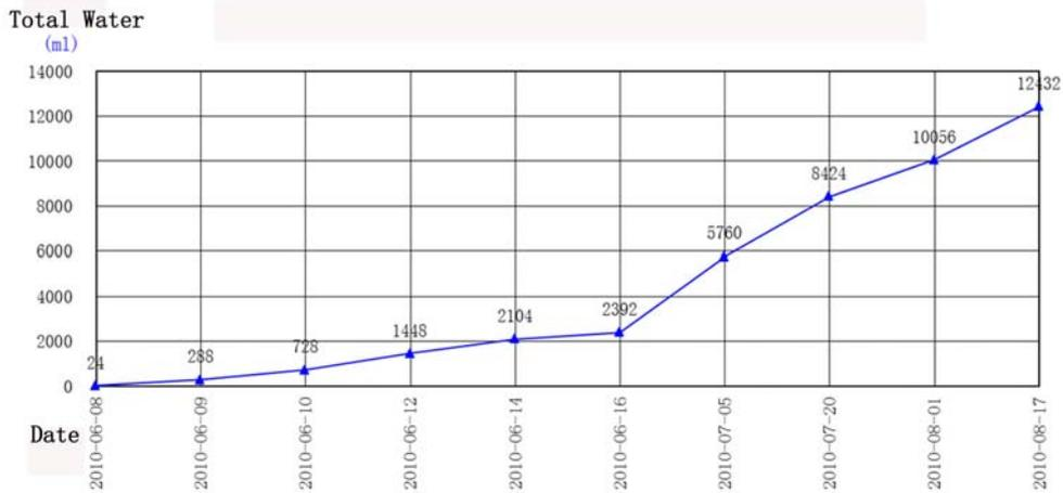
**Fig. 2** Aggregate flow curve of the water point 28.5m ahead of Roadway II5<sub>1</sub> (-720 m)
