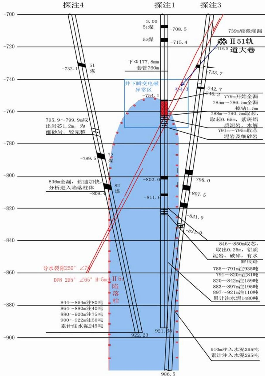
Fig. 6 Surface direction drilling-based delimitation of the concealed column (part)
