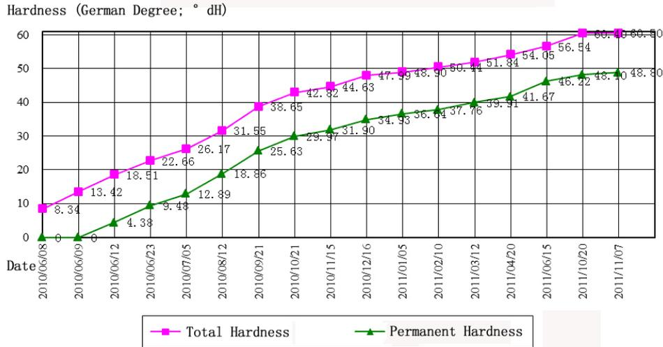
Fig. 4 Water hardness change curve of the water inrush points in Roadway II5<sub>1</sub>
