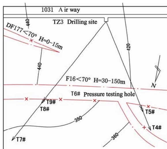
*Fig. 1 Plan of pressure water test*
