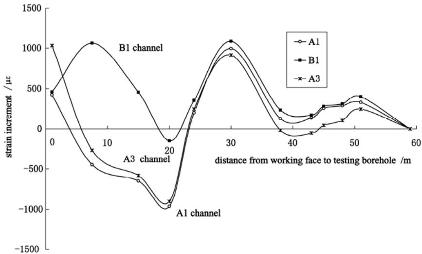
**Fig.5** The strain curves of field measurement in borehole of ventilation roadway
