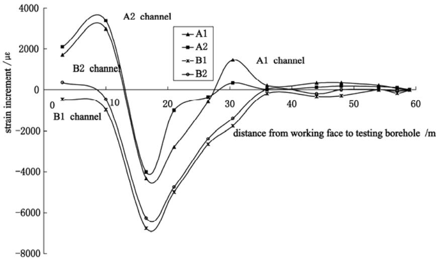
**Fig.6** The strain curves of field measurement in borehole of haulage roadway
