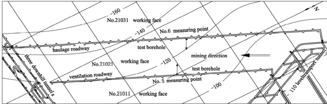
*Fig. 3 Schematic plane diagram of measurement borehole in roadway on 21021 working face*
