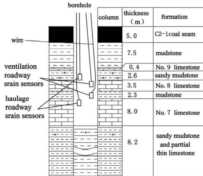
Fig. 4 Schematic diagram of the sensor laying strata in the borehole
