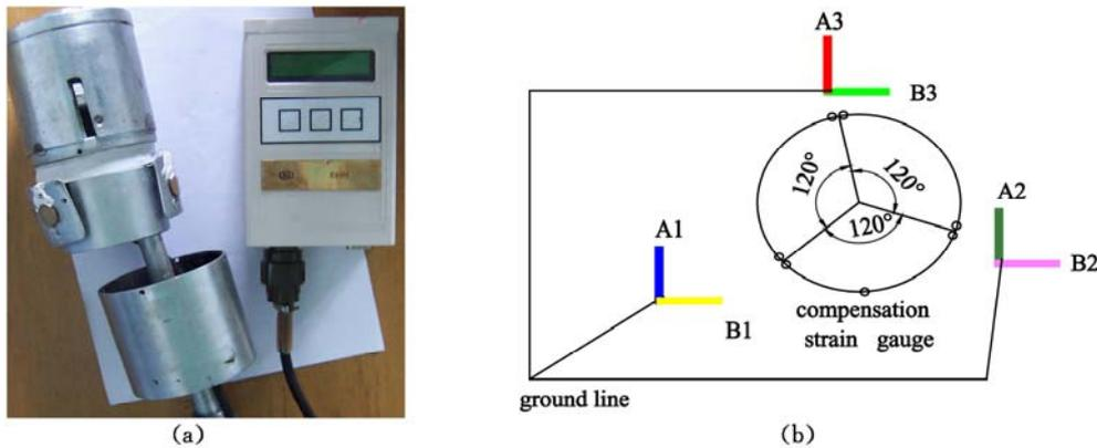
(a) Photos of sensor and strain recorder (b) Schematic of sensor's internal structure
