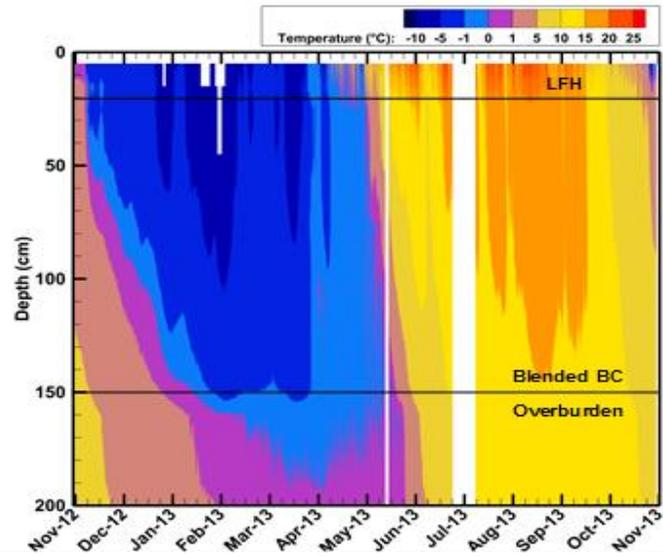
Figure 4 *In situ* soil temperature contours measured at Cell#18 (20 cm LFH cover treatment) during the 2012-
