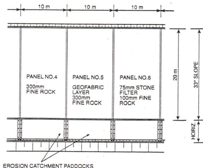
Figure 1 Part layout of erosion protection experiment
