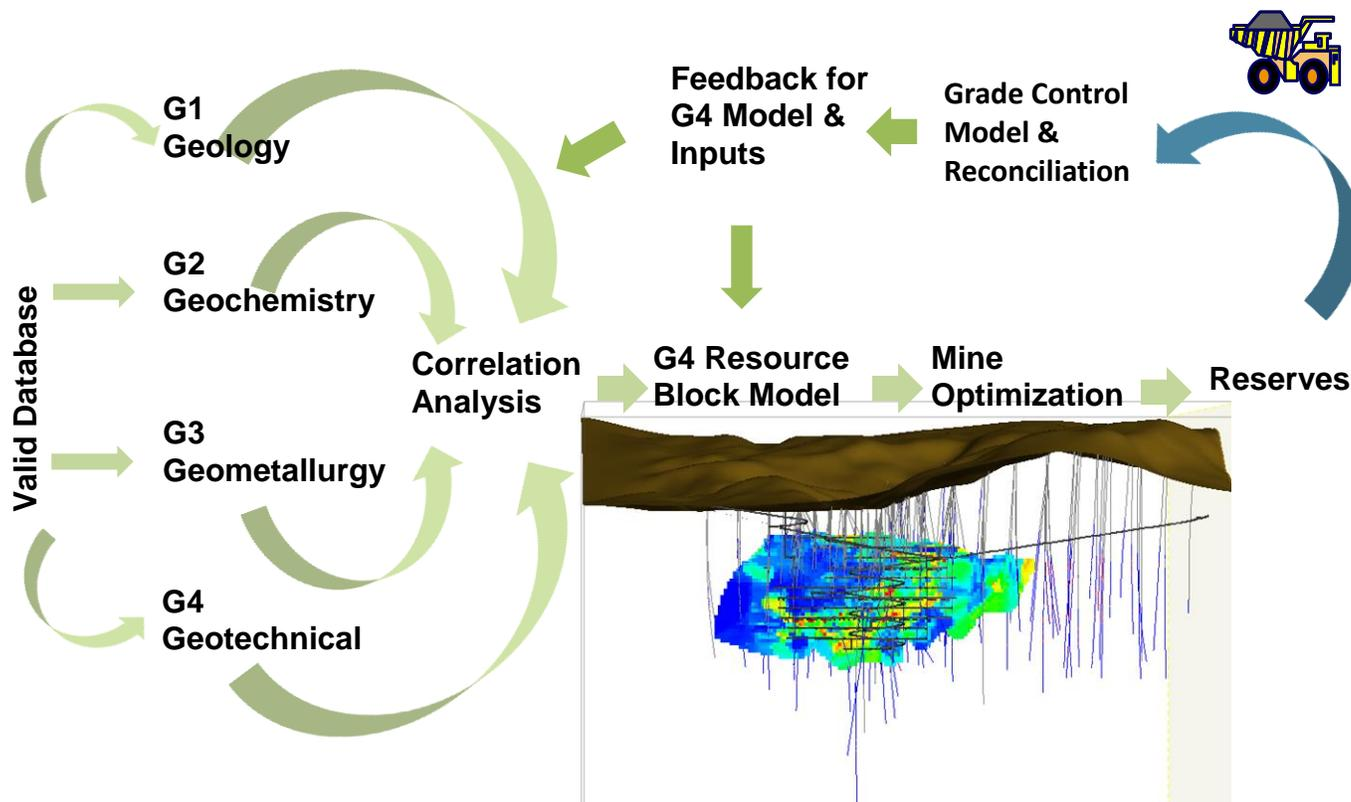
Figure 2 KGC G4 Process for Developing Resource Block Model and Mine Optimization
