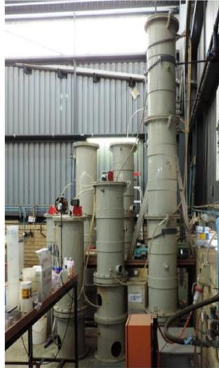
*Figure 2 Multi-stage column system used for test work*
