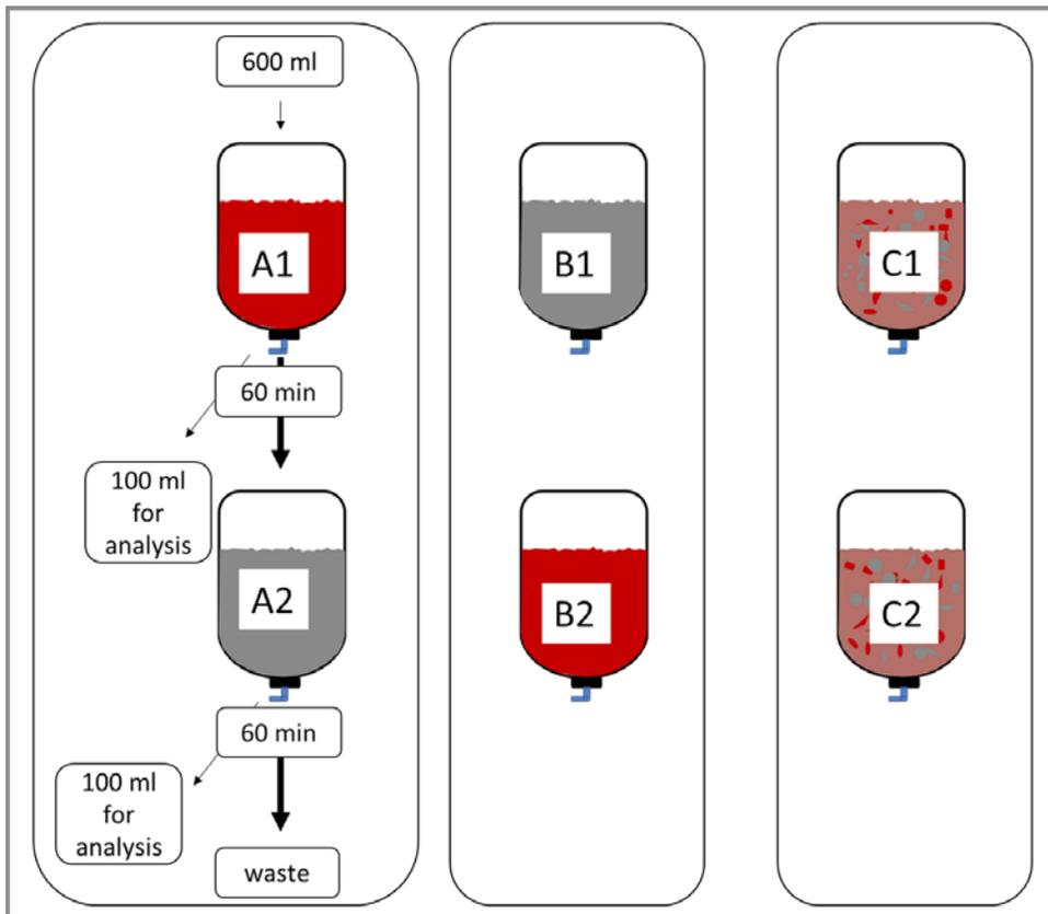
**Figure 4** Leaching systems –A, B and C. The sampling procedures described for system A applies for all three systems. Container A1 contains shale ash, A2 fines, B1 fines, B2 shale ash, C1 and C2 contain a mixture of shale ash and fines.
