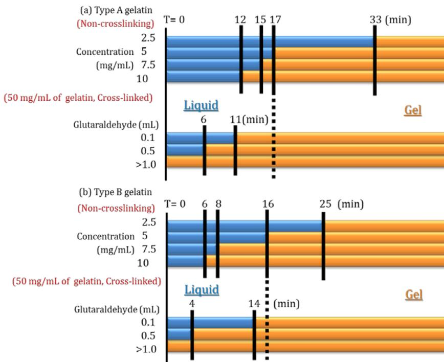
**Figure 1** Gelation time of Type A (a) and Type B (b) gelatin hydrogels with or without cross-linking at room temperature. Gelatin hydrogels with 5 mm thick were prepared in 8 cm square plastic dishes. Glutaraldehyde solutions were added to 50 mL of gelatin solutions
