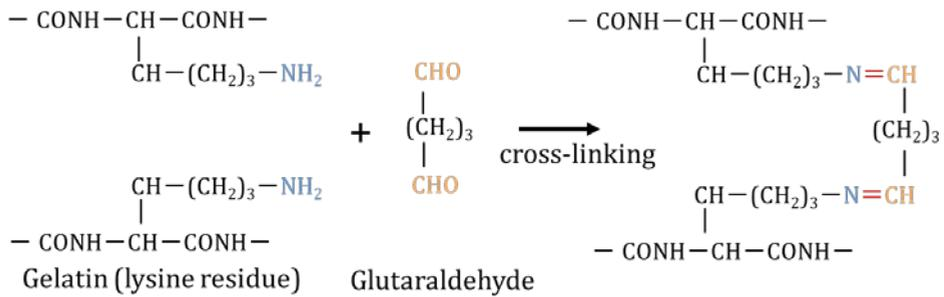
**Figure 2** Schematic illustration of cross-linking reaction between glutaraldehyde and gelatin.
