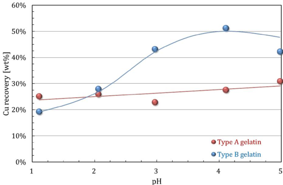
**Figure 5** Effect of pH on Cu recovery using cross-linked gelatin hydrogels. Cross-linked hydrogel sheets were prepared from 100 mg/mL of gelatin aqueous solutions
