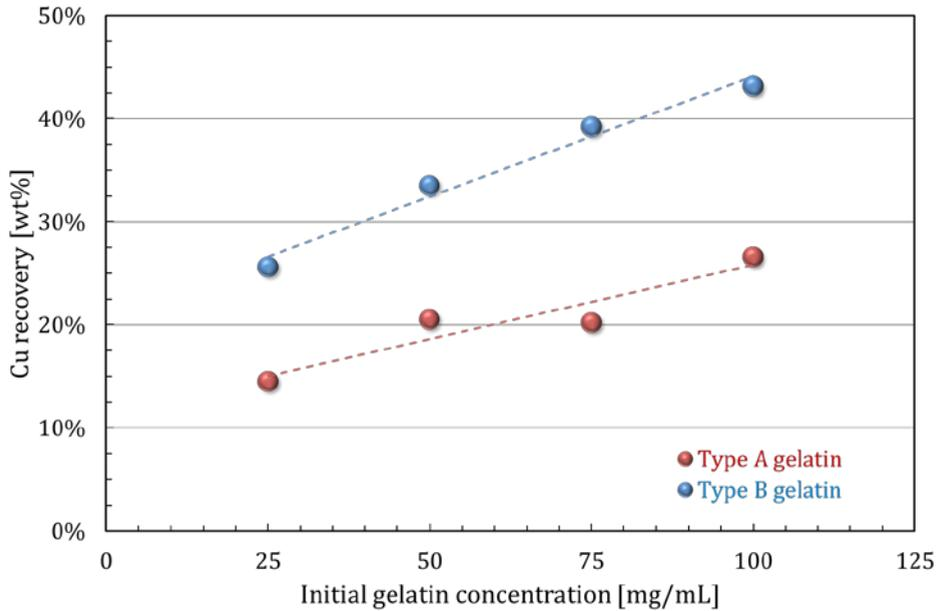
**Figure 4** Effect of initial gelatin concentration on recovery of Cu at pH 5. The initial concentration of Cu was 2 mM. Cross-linked hydrogel sheets were incubated in 10 mL of Cu solution at room temperature for 24 h.
