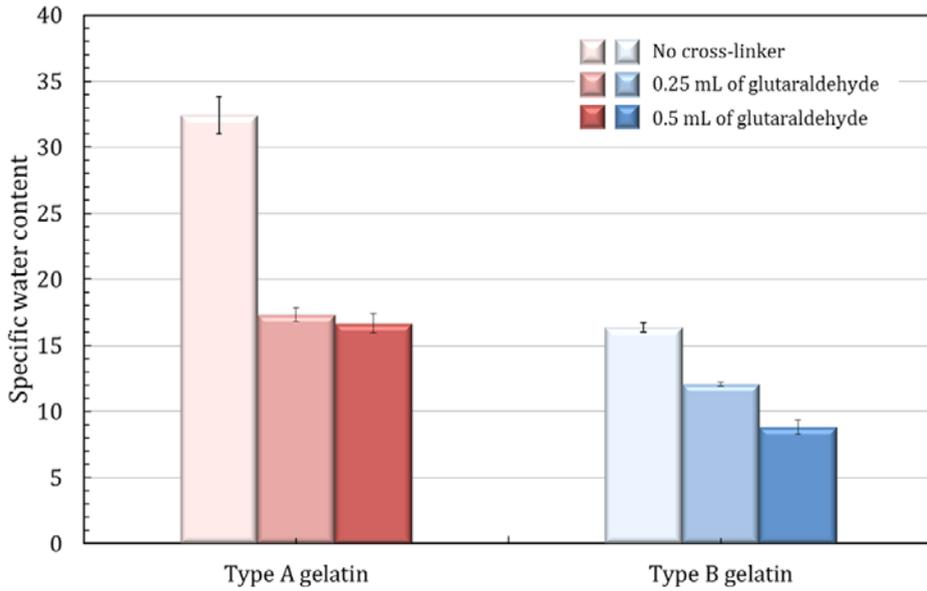
**Figure 3** Effect of addition of cross-linker on specific water content of Type A (a) and Type B (b) gelatin hydrogels. Glutaraldehyde solutions as a cross-linker were added to 50 mL of gelatin solutions
