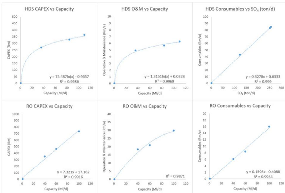
**Figure 3** Example CAPEX and OPEX relationships.
