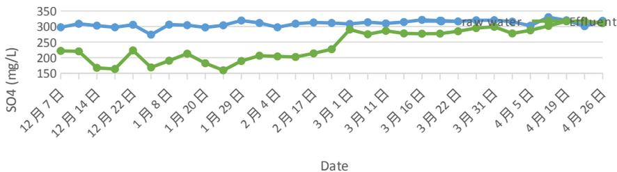
**Figure 3** Change in the Concentration of Sulfate Ion under the A-Condition
