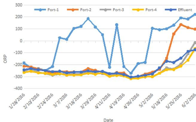
**Figure 5** Change in ORP in the Reactor under N-Condition
