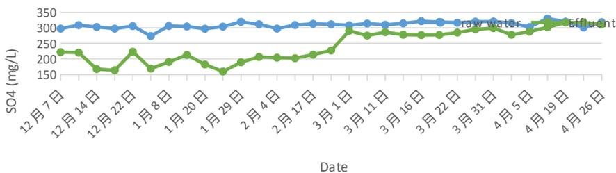
**Figure 3** Change in the Concentration of Sulfate Ion under the A-Condition
