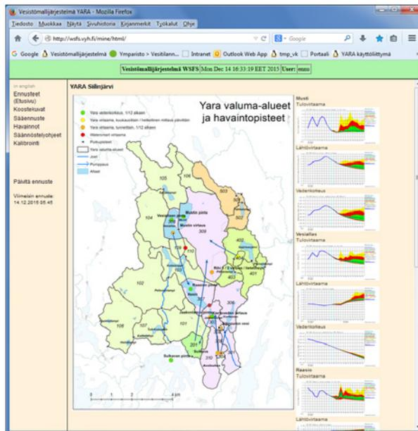
**Figure 2** Web interface for WSFS model. Clickable map shows the watershed description in the mining area and in some surrounding area. Clicking the map opens water balance pictures of the area. Some relevant graphs are on the right side of the map. Menu on the left side bar contains entries for entering observations, regulations schedules and discharge forecasts.
