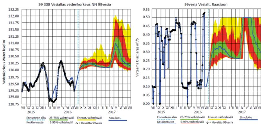
**Figure 3** Water level (on the left) and pumping (on the right) of Vesiallas pond are shown here as an example. Vertical dashed blue line shows the simulation date. Green, red and yellow bands on the right of it shows probability fractiles (50, 70, 90, 100 %) of forecasts.
