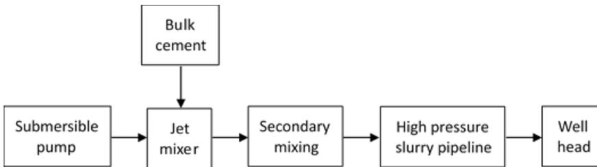
**Figure 3** Grouting process flow diagram.
