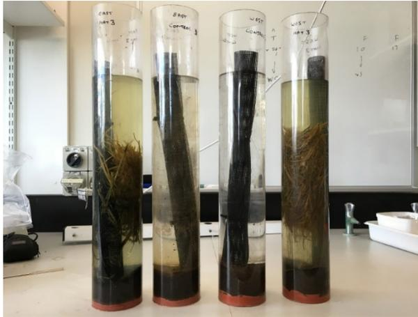
**Figure 1** Examples of microcosms, L to R: East Lake + hay, East Lake control, West Lake control and West Lake + hay, 14 days after hay was added (hay was later pushed down closer to the sediment).
