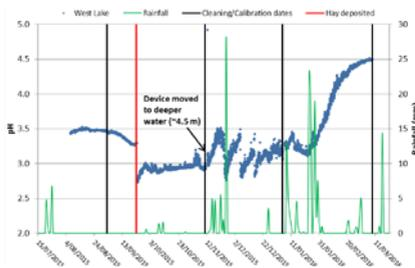
**Figure 2** pH changes in surface waters of a) East Lake microcosm, b) West Lake microcosm and c) West Lake (note probe moved from surface to ~4.5 m during experiment).
