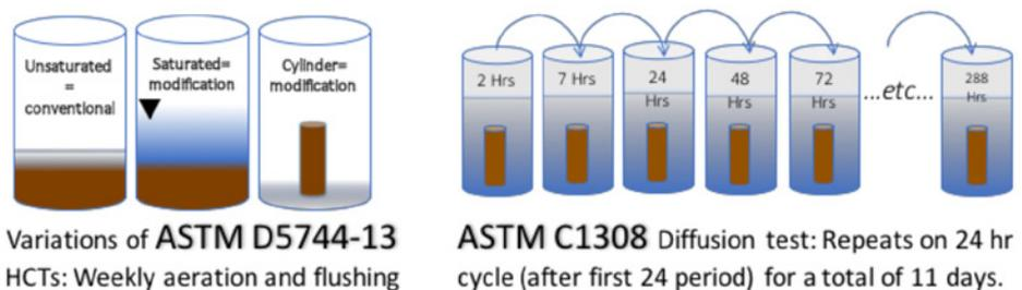
**Figure 1** Schematics of various test methods applied to evaluation of tailings management alternatives.
