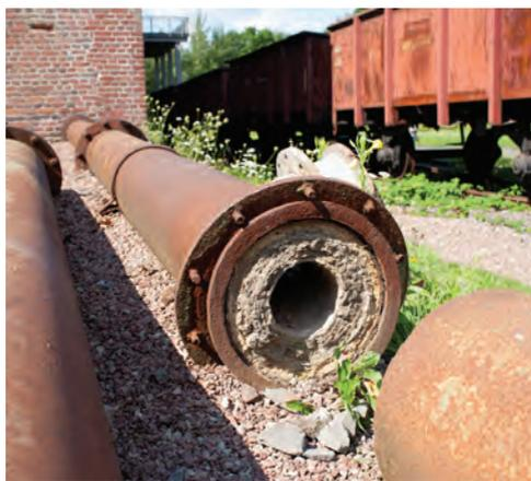
*Figure 2 A historical dewatering pipe of a former hard coal mine, Bochum shows the scaling potential of mine water (courtesy Felix Jagert).*
