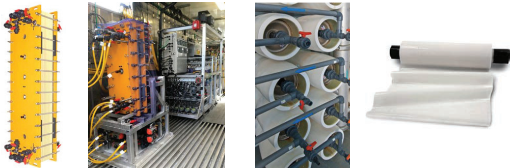
Figure 3 (left to right) Salt Splitting Stack, ED-RO pilot, RO elements, and salt splitting ion exchange membrane
