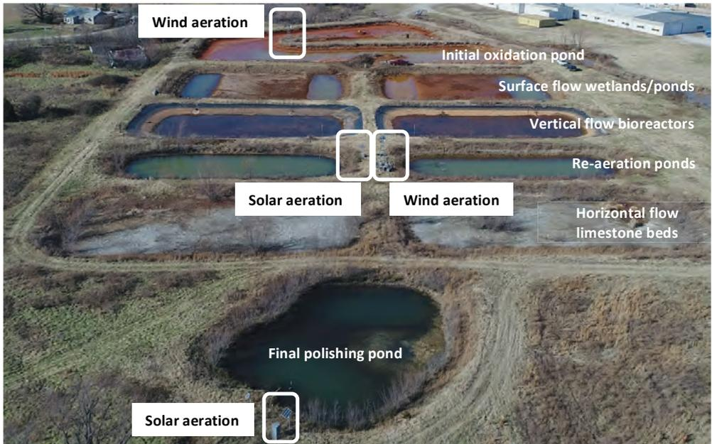
*Figure 1 Oblique aerial photograph of Mayer Ranch passive treatment system in December 2017 during a maintenance drawdown when water levels were decreased. Water flow paths are from top to bottom. Individual process unit designations and locations of aeration devices are shown. Image obtained via small Unmanned Aerial System.*
