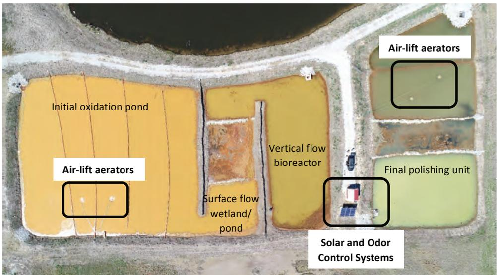
*Figure 2 Vertical aerial image of Southeast Commerce passive treatment system in April 2018. Individual process unit designations and locations of aeration and other devices are shown. Note directional baffle curtains in the initial oxidation pond. Image obtained via small Unmanned Aerial System.*
