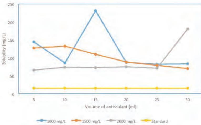
*Figure 5 Effect of various volume of antiscalant on CaCO<sub>3</sub> dissolution*
