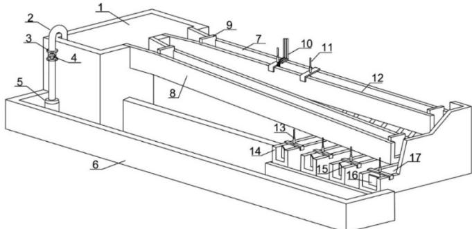
*Fig.1 The experiment device of water insush: 1 Reservoir; 2 Water supply pipes; 3 Flange; 4 Valve; 5 Water pump; 6 Backflow pool; 7 Leaky sink(1); 8 Leaky sink(2); 9 Movable baffle; 10 Pitot tube; 11 Movable needle detector; 12 Changeable crack; 13 Fixed needle detector; 14 Backflow channel; 15 Triangular weir; 16 Rectangle weir; 17 Backflow channel; 18 Steady flow velocity grilling*
