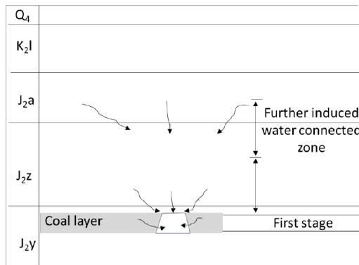
Figure 1 schematic map of hydrogeologic condition shifting at the Xiaojihan col mine
