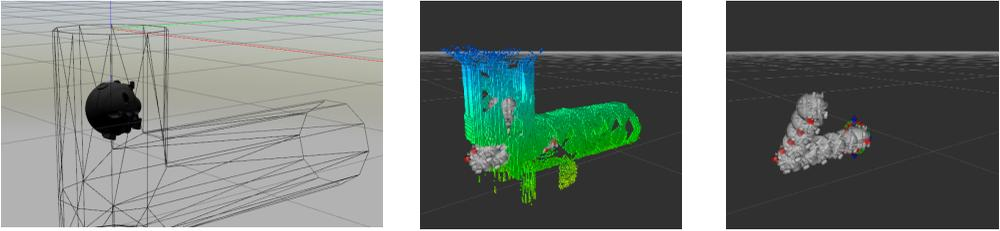
**Figure 6** Example of trajectory planning (a) Current position of the robot (b) Built map and the planned trajectory (c) View without the visualization of the map.
