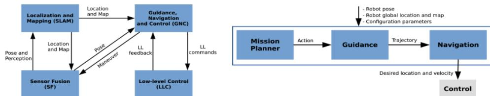
Figure 2 (a) Robot software architecture and (b) Simplified diagram of the GNC module.
