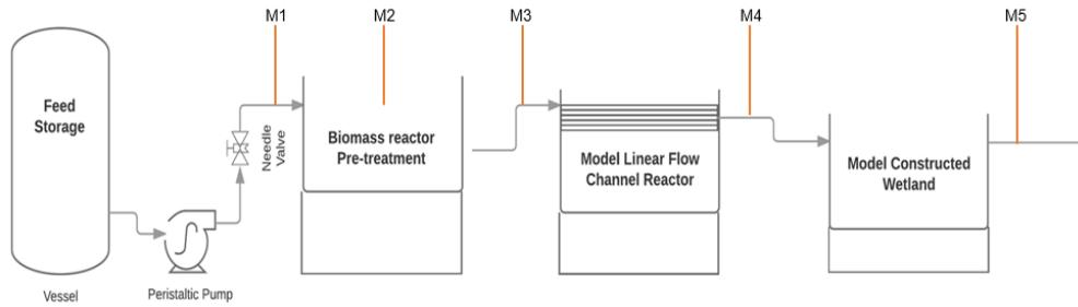
Figure 1 Layout of the model continuous system with liquid sampling points indicated (M1 to M5)
