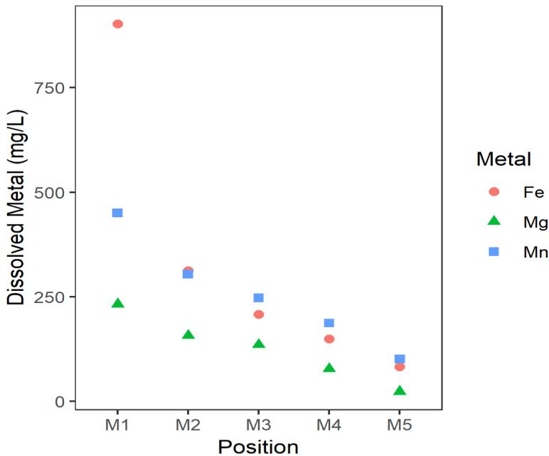
Figure 6 Snapshot of some metal concentrations at 96 hours for the model continuous flow series as laid out in Figure 1 with a 48hr hydraulic retention time relative to the LFCR
