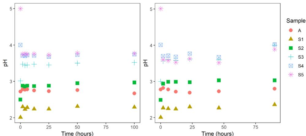
Figure 2 pH change for dilutions of Sulfuric acid contacted with 15g (left) and 25g (right) of Sugarcane Bagasse
