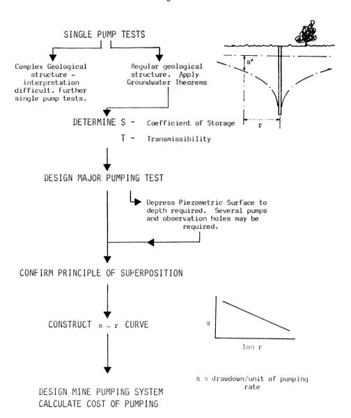
Fig. 1. Pumping System Design Proceedure
