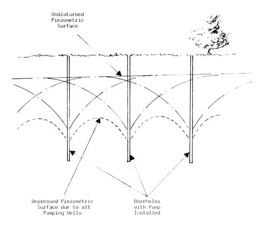
Figure 2. The Principle of "Superposition"
