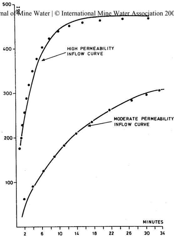
Figure 1 Simulation of DST inflow data
