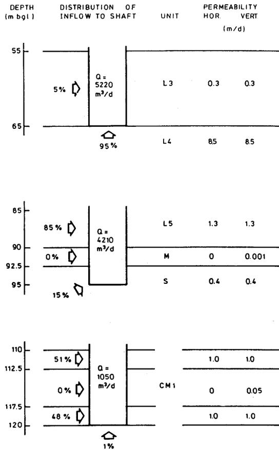
Figure 5 Distribution of inflow over sides of shaft open section at depths of 65 , 95 m and 120 m
