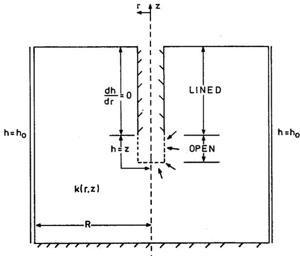
Figure 2 Definition sketch of vertical section through flow domain of a shaft inflow problem.
