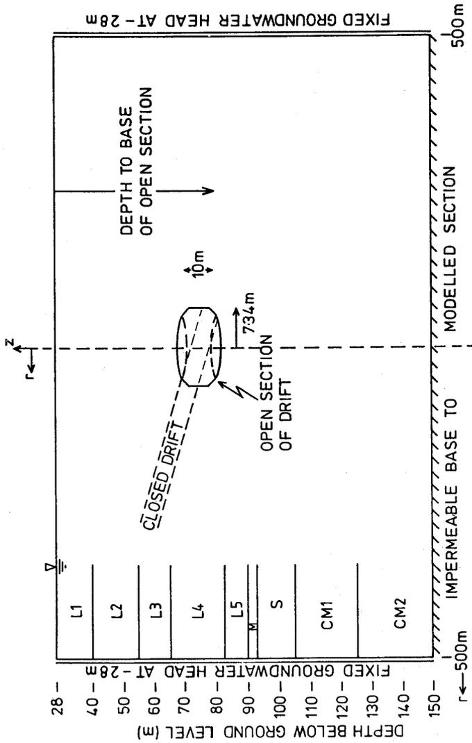
Figure 9 Vertical section through flow domain showing representation of drift open section
