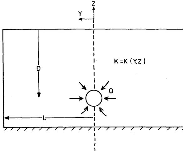
Figure 7 two dimensional approximation for drift inflows
