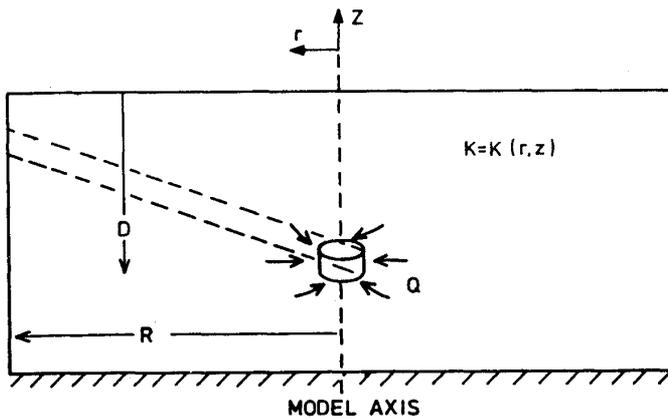
Figure 8 Radial (r-z) approximation for drift inflows
