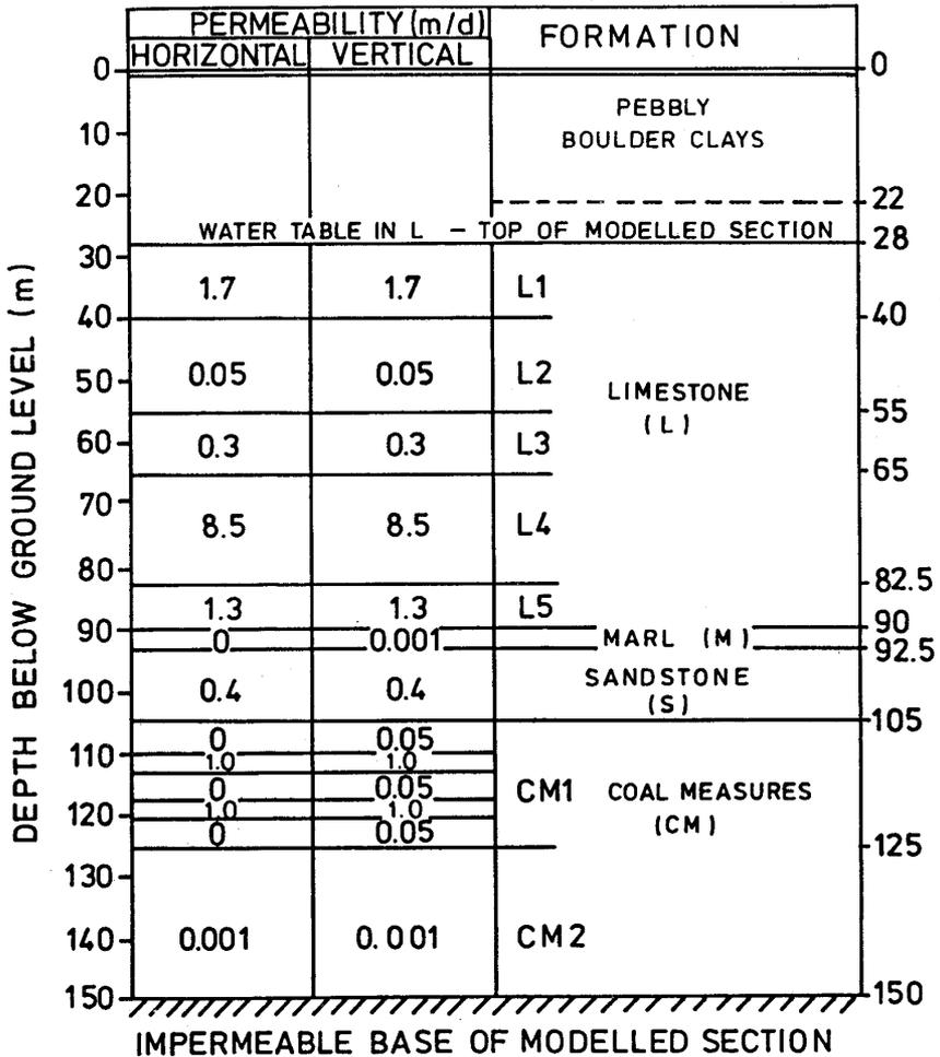
Figure 3 Permeability depth-profile for shaft and drift inflow estimation
