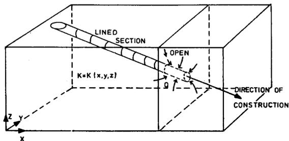
Figure 6 Three-dimensional inflows of a drift
