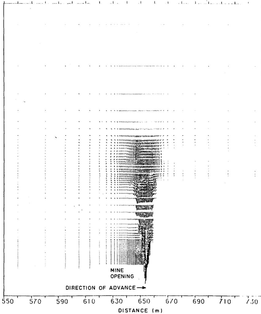
Figure 11 Flow distribution to a longwall face
